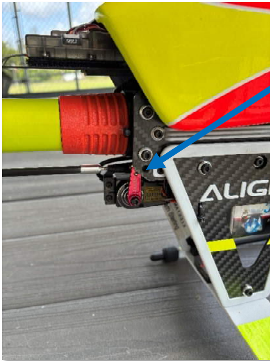
Photo #4- A typical servo arm at neutral with about 90 degrees to its pushrod.
