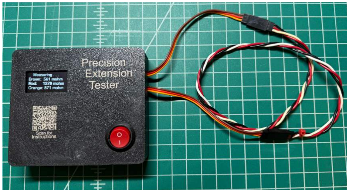
Very high resistance shows a bad cable
