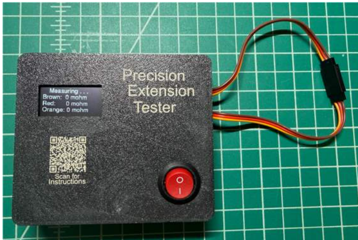
The new tester finished self-calibration
