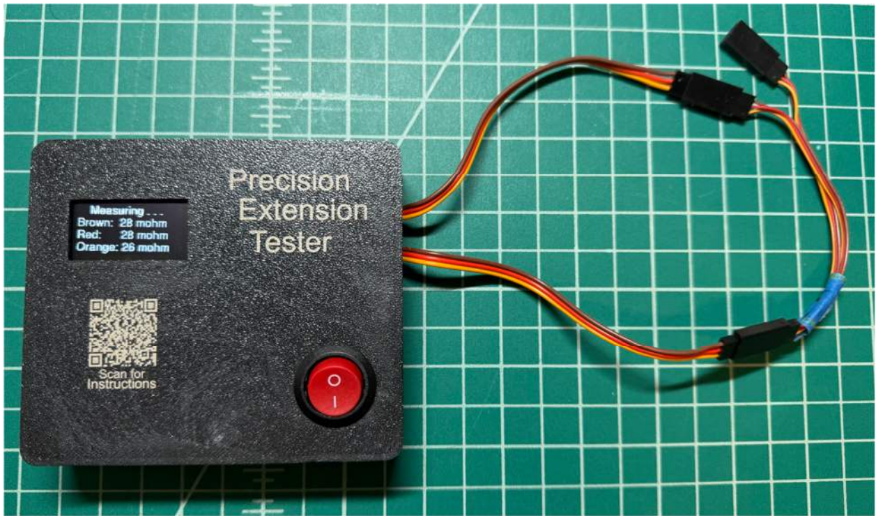
e-Flite Y-cable looks good with low lead resistance
