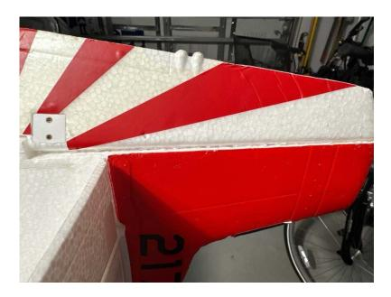
Here is the new hinge line for the rudder. After watching the video, I may return to touch up the hinge. A Q-tip with Foam-Tac would smooth out the hinge line.
