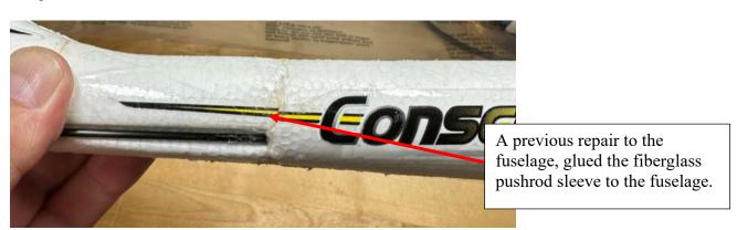
It took a crash to find the problem. Post-crash, the plane functioned properly, or so I thought. It wasn't until I had the plane on the bench that I found the two servos had almost no power to move the elevator and rudder...shocking. I disconnected the linkage at the tail surfaces and flexed both the rudder and elevator looking for the source of stiffness, but both moved freely, or as free as a foam hinge surface can move.
