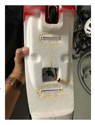
All the gear was reinstalled in the Fuselage, servos, receiver, motor, ESC and nose gear. Surprisingly, no servos were stripped. The receiver was secured with some silicone adhesive. It's possible the original adhesive failed here and the AS3X receiver broke free, causing the crash. It's solid this time.
